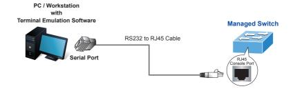
Figure 4-1: Managed Metro Switch Console Connectivity
