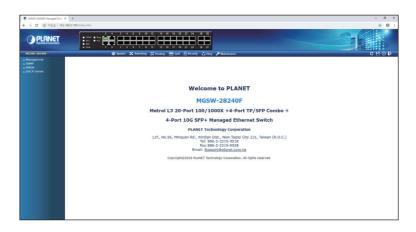
Figure 5-3: Web Main Screen of Managed Metro Switch
